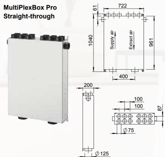
The standard 2x6 sets of Supply and Extract AirflexPro connections are orientated to give straight through duct connections. 1x extra port for supply and extract is located on the side of the unit. These are facilitated by knockout points. Compact design with easy installation and maintenance. Please see above image for the individual dimensions. Unit supplied with two inspection covers, one on each side enabling the unit to be left or right handed.
