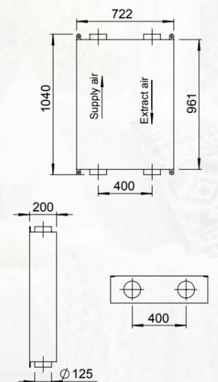
Standard 4x 125mm Ports are placed at the top and bottom of the item to give straight through duct connections. Compact design with easy installation and maintenance. Please see above image for the individual dimensions. Unit supplied with two inspection covers, one on each side enabling the unit to be left or right handed.
