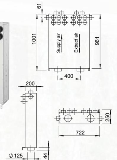
The standard 2x6 Supply and Extract AirflexPro connections are orientated 90 degrees to the main body. 1x extra port for supply and extract is located on the side of the unit. These are facilitated by knockout points. Compact design with easy installation and maintenance. Please see above image for the individual dimensions. The supply air to the dwelling is on the left hand side in this unit as you look at the unit.
